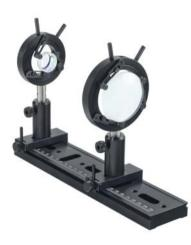
Simple lenses are subject to optical aberrations. In many cases these aberrations can be compensated for to a great extent by using a combination of simple lenses with complementary aberrations. A compound lens is a collection of simple lenses of different shapes and made of materials of different refractive indices, arranged one after the other with a common axis.
